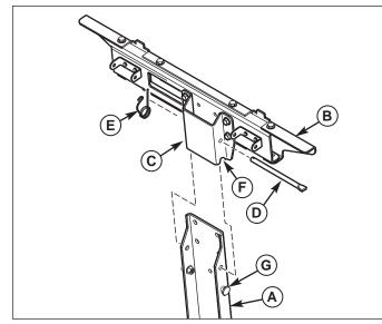
Figure 3. Install Bag and Cover Support
